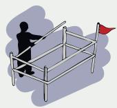
Preparing to cut a deck opening: protection railing is installed prior to steel cutting removal.
